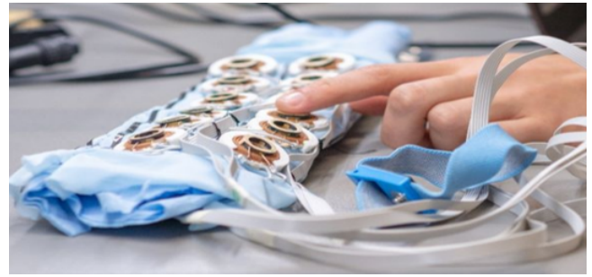
Figure 4: The vibration motor array of the prototypical haptic sleeve
